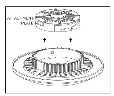
**Step 2:** Securely attach and tighten the Light Kit Attachment Plate to the bottom of the ceiling fan motor by routing the wires through the Attachment Plate and then lifting the Light Kit Attachment Plate and screwing onto the motor shaft, hand tightening only.
