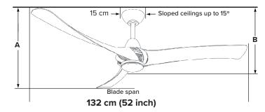
A: 33 cm CEILING TO BOTTOM OF MOTOR B: 30 cm CEILING TO BOTTOM OF BLADES
