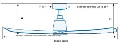
132 cm (52 inch) A: 32 cm CEILING TO BOTTOM OF MOTOR CEILING
