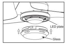
**9.** Secure the glass to LED plate by twisting in in a clockwise direction. Do not over-tighten.
