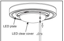
**4.** Disassemble the LED clear cover from the LED plate by removing three screws and retain the removed screws for Step 8.
