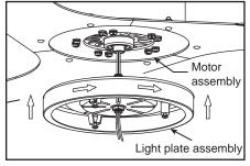
**3.** First pull out light wire lead and remove the shrinkable sleeve then through the hole in the light plate assembly. Assemble the light plate assembly to the motor assembly by twisting in a clockwise direction until tight.
