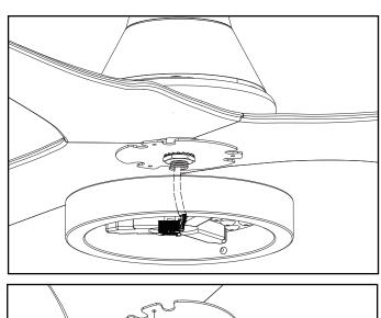
**Step 2:** Securely attach and tighten the Light Kit Fixture onto the Flxing Steel Plate using the 3 screws provided.
