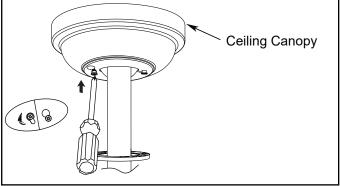
**Step 2:** Securely attach and tighten the ceiling canopy screw cover over the shoulder screw heads in the hanger bracket utilising the key slot twist-lock feature.
