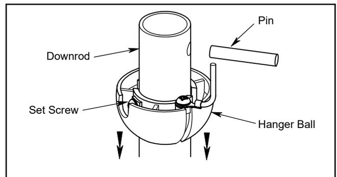
**Step 2:** Remove the Hairpin Clip and Clevis Pin from the bottom of the Downrod. Retain the pin and clip for reinstallation in Step 4.
