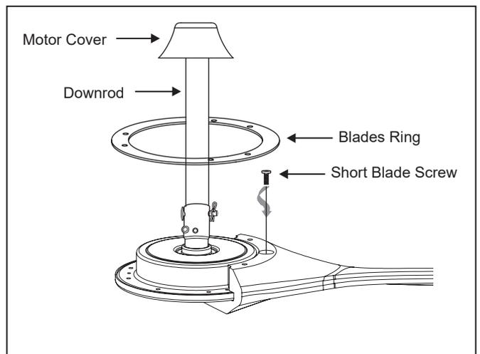
**Step 2:** Slide the Blades Ring down over the Downrod and onto the Blades, aligning the holes in the Blades with the holes in the Blades Ring. Install the two long blade screws into each Blade through the Blade Ring.
